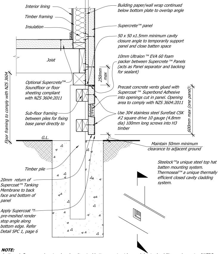
As the sub-floor space is not a closed cavity, steel battens must not be used due to durability requirements of NZBC. Instead, fix the sub-floor cover panel directly to timber framing. As this is potentially damp, H3 treated timber, stainless steel wood screws 100mm long at 600mm centres must be used
